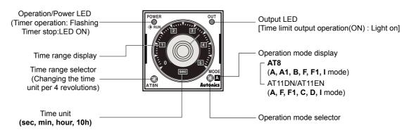
XPlease rotate the time range switch and operation mode switch to CW(Clockwise) direction.
